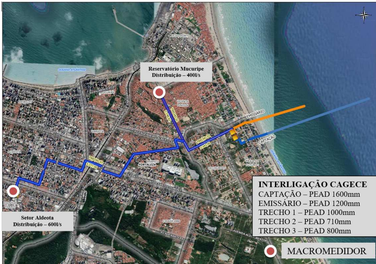
Figure 10.1 - Intake System Scheme Configuration
