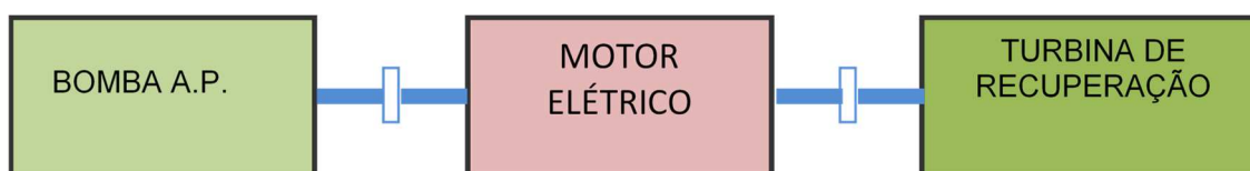
Figure 4.18 - Brine Energy Recovery System by Turbine in an RO Plant
