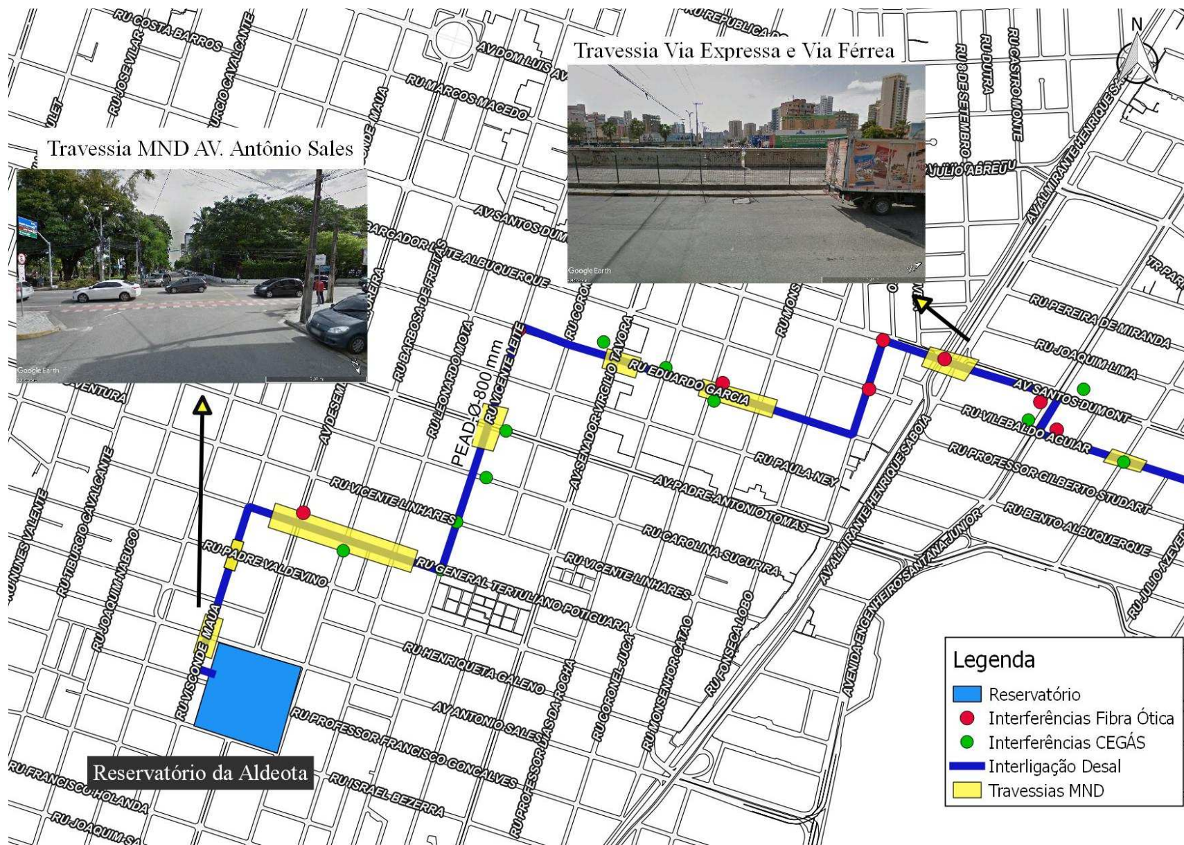
Figure 2.6 – Interferences of the Interconnection Water Main with the Existing System
